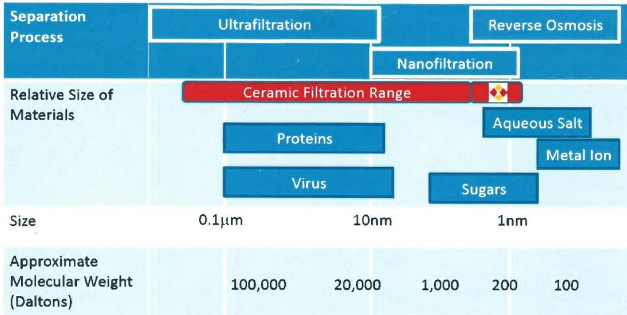
Figure 1: Ceramic filtration ranges<sup>1</sup>
