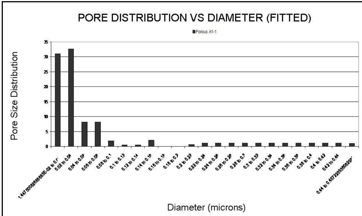
Pore size distribution of Porous A1-1. A similar distribution can be expected for all A1 class materials, albeit with different bubble points.
